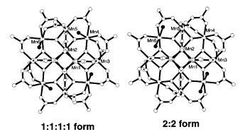
**Figure 1.** [Mn<sub>12</sub>O<sub>12</sub>(O<sub>2</sub>CC)<sub>16</sub>O<sub>4</sub>] core structures of two water isomers, the 1:1:1:1 form and the 2:2 form, in 2a·2H<sub>2</sub>O. The isomers result from the disordering of two carboxylates out of 16. Oxygen atoms of water molecules are indicated by filled circles.
