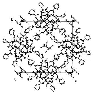
Figure 2. Molecular packing of 2a·2H<sub>2</sub>O viewed from the c-axis. Hydrogen and fluorine atoms and water oxygen atoms incorporated into the crystal were omitted for clarity.
