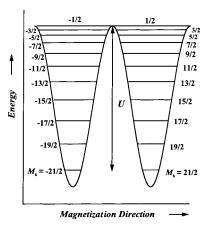
**Figure 6.** Plot of potential energy vs the magnetization direction for a single molecule with a  $S = {}^{21}/{}_2$  ground state split by axial zero-field splitting. The potential energy barrier U is given by 110|D|.
