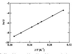
**Figure 7.** Plot of the natural logarithm of the magnetization relaxation rate  $[\ln(\tau)]$  vs the inverse of the absolute temperature for complex 2a- $2H_2O$ . The solid line represents a least-squares fit of the data to the Arrhenius equation (see text).
