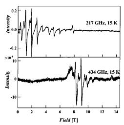
**Figure 11.** HFEPR spectra for a microcrystalline sample of complex **2a**·2H<sub>2</sub>O recorded at 217.23 GHz (top) and 434.24 GHz (bottom) for temperature 15 K.
