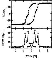
**Figure 13.** Top: Magnetization hysteresis loop measured at 1.85 K for microcrystals of  $2c \cdot 2CH_2Cl_2 \cdot C_6H_{14}$ . Samples were oriented in eicosane wax matrixes. Bottom: The first derivative of the magnetization hysteresis loop.
