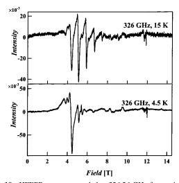
**Figure 10.** HFEPR spectra recorded at 326.26 GHz for a microcrystalline sample of complex **2a**•2H<sub>2</sub>O that had been oriented in a strong field. The top plot is of the 15 K spectrum, whereas the 4.5 K spectrum is shown in the bottom plot.
