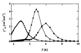
**Figure 8.** Ac out-of-phase signals  $(\chi''_M)$  of  $[\text{Fe}(C_5\text{Me}_5)_2]_n[\text{Mn}_{12}\text{O}_{12}(\text{O}_2-\text{CC}_6\text{F}_5)_16(\text{H}_2\text{O})_4]$   $(n=0,\ 2\ (\blacksquare);\ n=1,\ 2a\ (\bullet);\ n=2,\ 2e\ (\blacktriangle))$ . The lines are visual guides.
